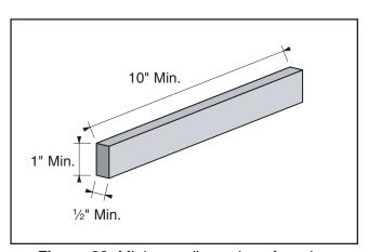
**Figure 20.** Minimum dimensions for edge jointing.
